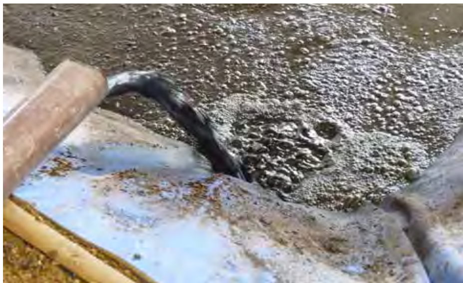
Figure 21. Observe the color of the discharge. Black or very dark brown or grey is normal. Any other color could indicate industrial pollutants.
