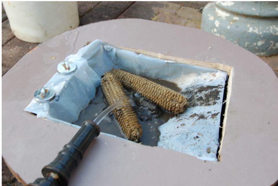
Figure 6: Overall view of the dumping basin with its plywood base. The basin is lined with a Teflon sheet to simulate the fact that ultimately the basin would be made of molded Teflon to resist things sticking to it. In the basin is some potting soil and water is being added to start the dumping process. The water could be the waste water from a hand washing station.
