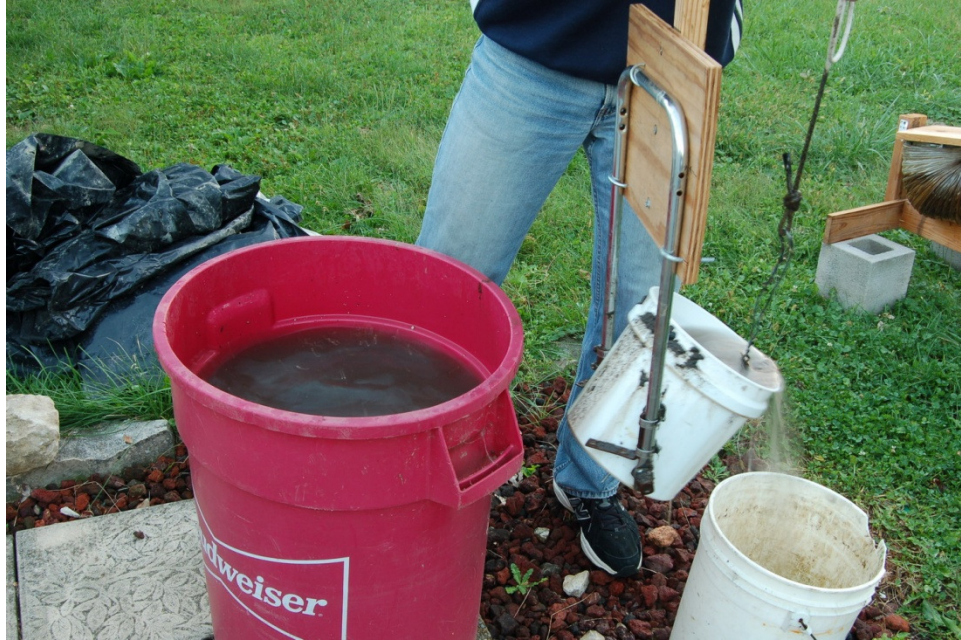
Figure 3: By lowering the rope (in the user's left hand) while holding the handle (in the user's right hand) the bucket is dumped into a receiving vessel for transport.
