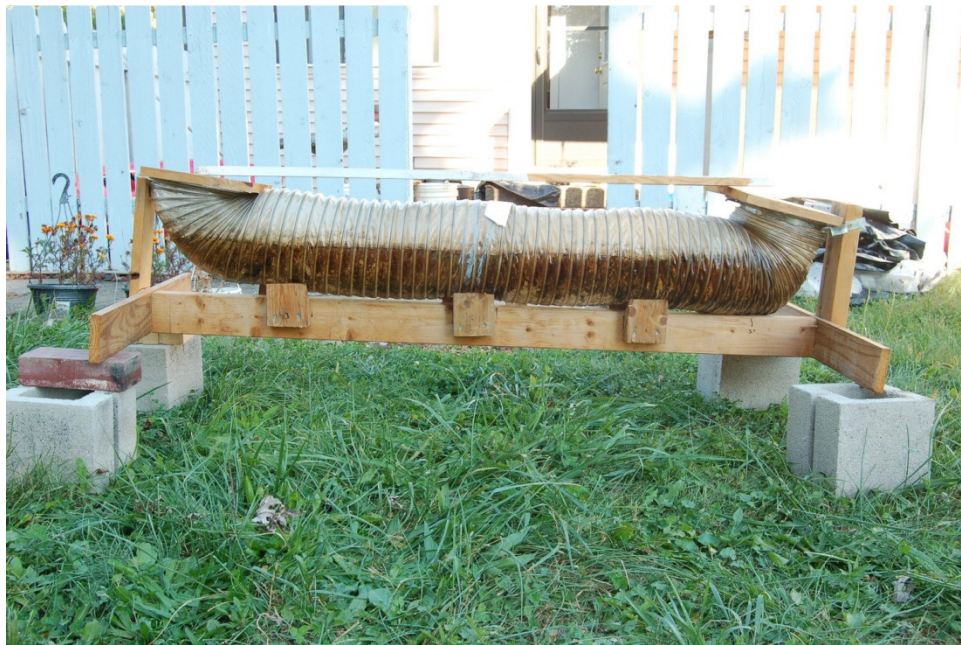
Figure 11: Tube pasteurizer without the cover. The inlet end is the high end on the left, with the outlet on the right.
