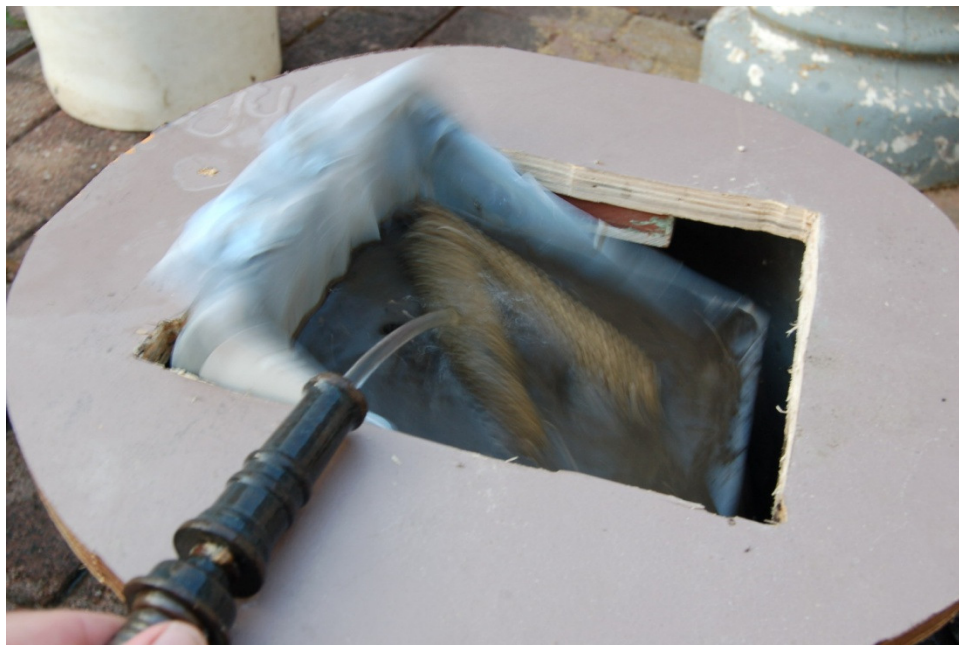
Figure 8: The basin in the process of tipping. The contents are quickly dumped out the right side of the basin into the chamber below.
