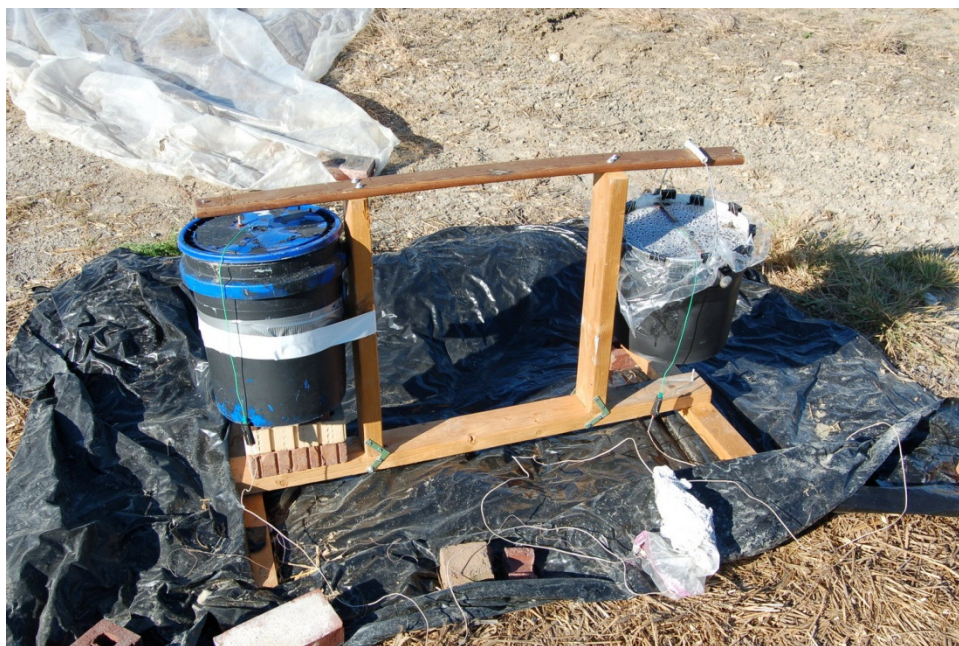
Figure 10: The bucket pasteurizer with the top cover removed. There are two buckets present, the one on the left holds about 19 liters but it only 80% full. The one on the right holds about 15 liters and is full.
