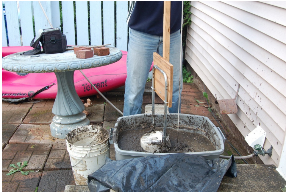
Figure 4: The system is being used in thicker material. Here, the rope is completely lowered so that the bucket is completely upside down. It is then pushed down into the material, while gently sweeping from left to right. This requires light force, usually not much more than the weight of the system. The bucket has a stop which prevents it from rotating past the fully down position.
