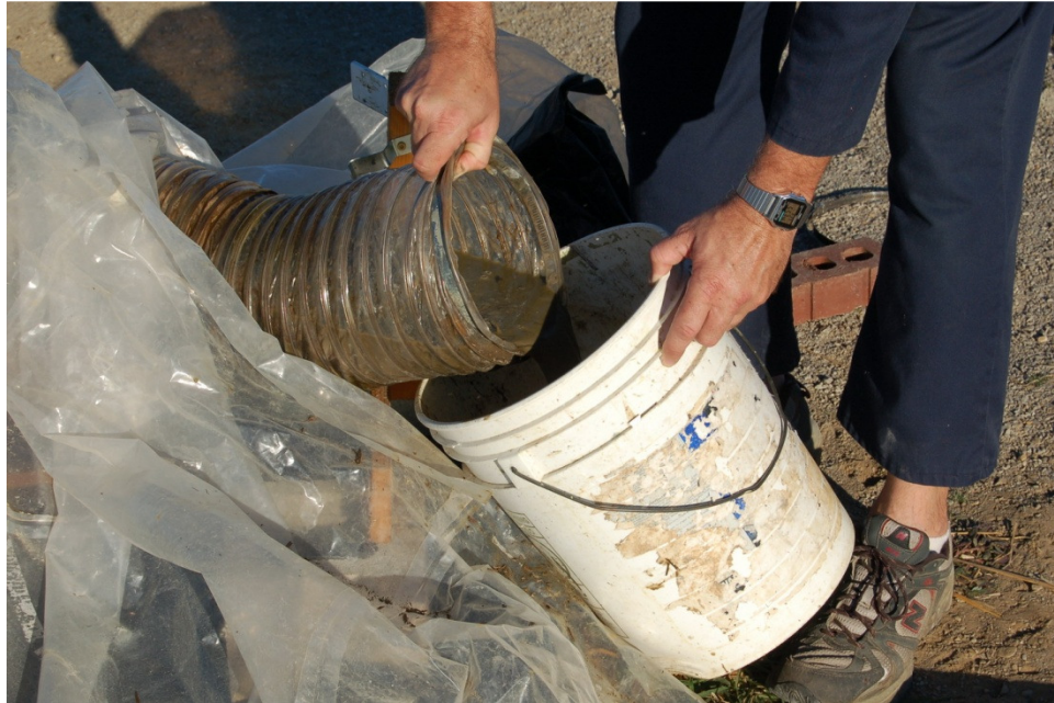
Figure 13: Emptying the tube pasteurizer. The small handle is hidden inside the operator's hand. The portion of the tube being touched by the operator is never in contact with feces, and is therefore should be clean. A better handle will be developed and will completely eliminate any possible contact.
