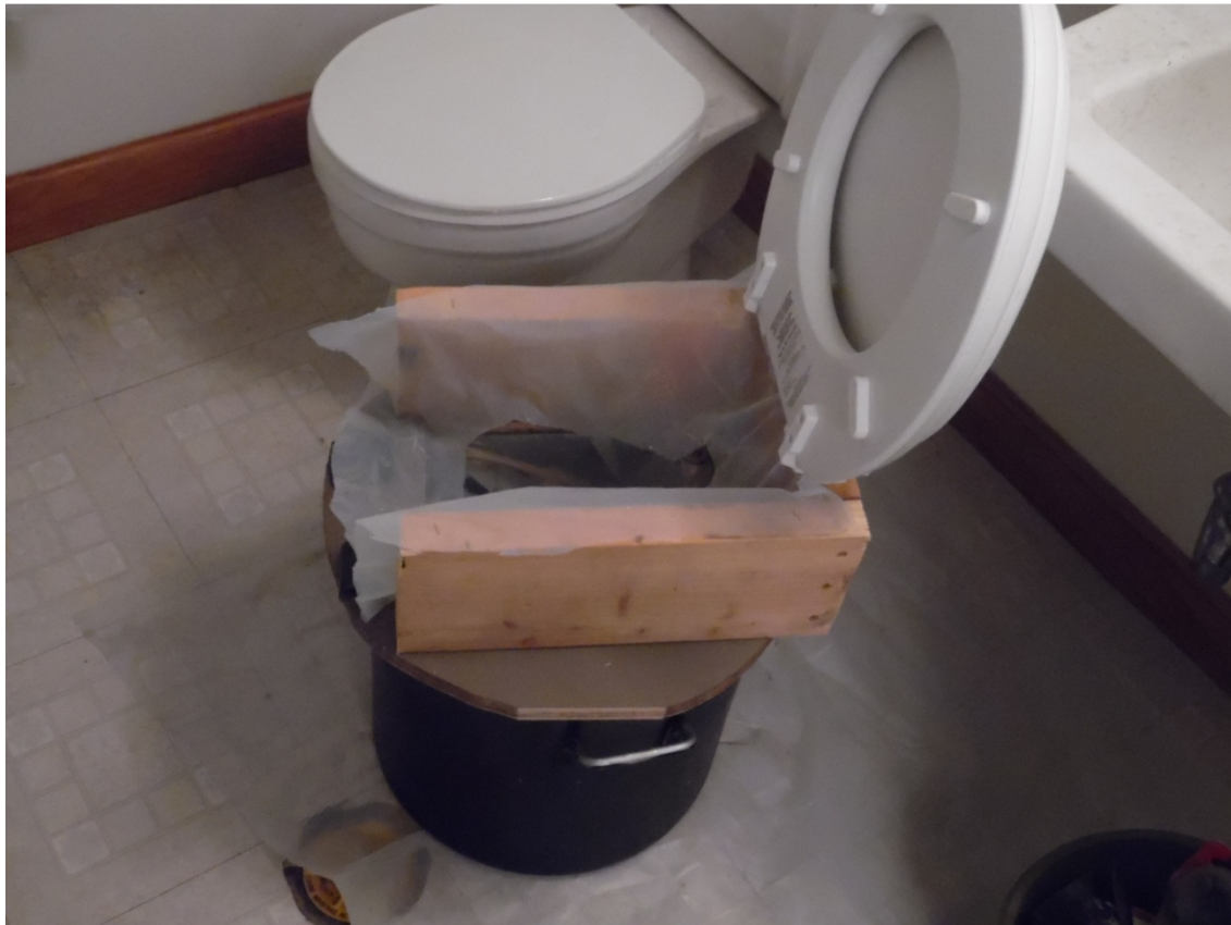
Figure 9: The dumper assembled into a fully functional toilet. This unit was used for a week by the author, with good results.
