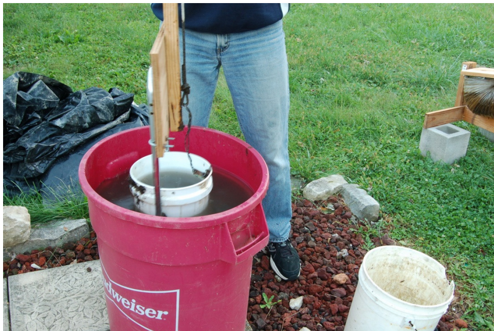
Figure 2: The bucket loaded with liquid, ready to be pulled out of the pit.
