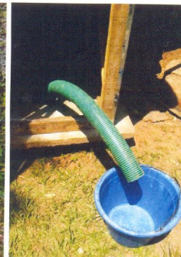
The suction hose pipe makes the pit emptying operation cleaner.
