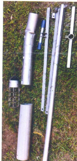
The rammer can be disassembled for tranquil cleaning and transportation.
